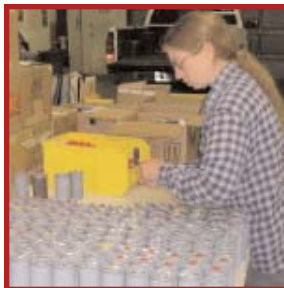
On the assembly side, grenades are cleaned, inspected and identified by lot number.
