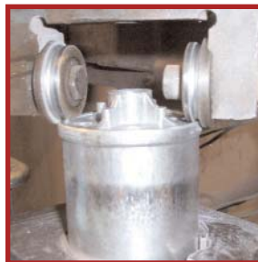
The igniter formulation is added and a lid is securely rolled on top of the canister.
